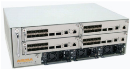
Figure 4. The Aruba 6000 Controller supports up to 8,192 RAPs.
