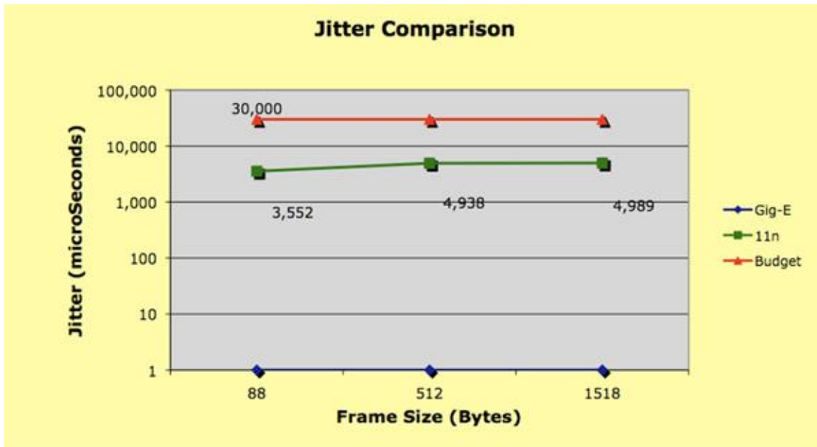
Figure 3: Jitter: Gigabit Ethernet vs. 802.11n (Source Data: Network World tests)
