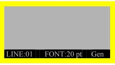
The display allows you to see up to three lines of text and 16 characters per line. The display auto-scrolls when you enter more than the maximum displayed lines or characters. Use the arrows on your keypad to navigate the screen.
